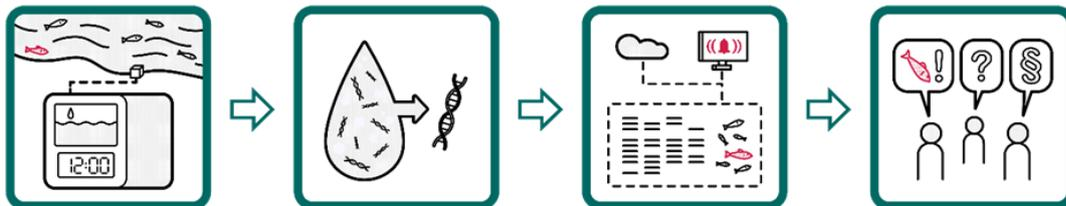
Figure 1. Illustration of the various steps in automatic environmental monitoring. The first image shows a continuous collection of samples from water. Then the samples are processed, and DNA is extracted. Finally, the samples are analysed, and warnings are sent if anything undesirable is detected. Such a facility will allow early action to limit and prevent damage.
