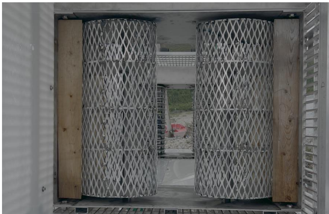
Figure 3. Modified entry gates to the sorting platform, with some plates removed and gates covered by wire mesh.
