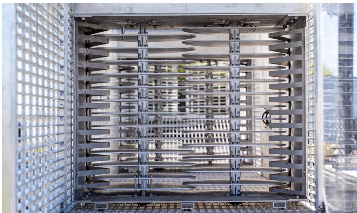
Figure 2. Original entry gates to the sorting platform, consisting of stacked, rotating plates.
